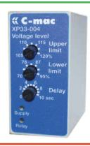
The C-mac<sup>®</sup> module type XP33-004 monitors its own 3-phase supply voltage, and checks that all 3 phase-neutral voltages are within the adjusted limits, and in that case, the output relay is activated.
